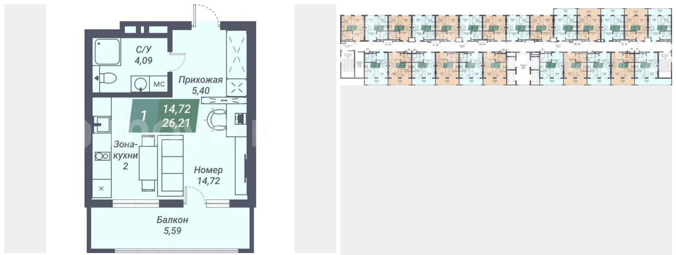
The top left image shows a detailed floor plan of an apartment unit. The layout includes a bathroom (C/У 4,09), a walk-in closet (МС), a hallway (Прихожая 5,40), a kitchen (Зона-кухни 2), a living room (1 14,72), a balcony (Балкон 5,59), and a bathroom (Номер 14,72). The total area is 26,21 square meters. The top right image is a long horizontal diagram showing the layout of multiple floors or units in a building, with various rooms and hallways labeled.
